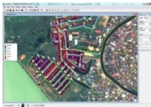
Figure 2. The Pipe Network System in Taman Khayangan Resident Makassar by using the EPANET 2.0 Software.
